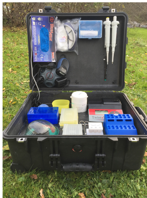
Fig. 1. Diagnostics-in-a-Suitcase. It contains all equipment and reagents for performing the RT-RPA assay.
