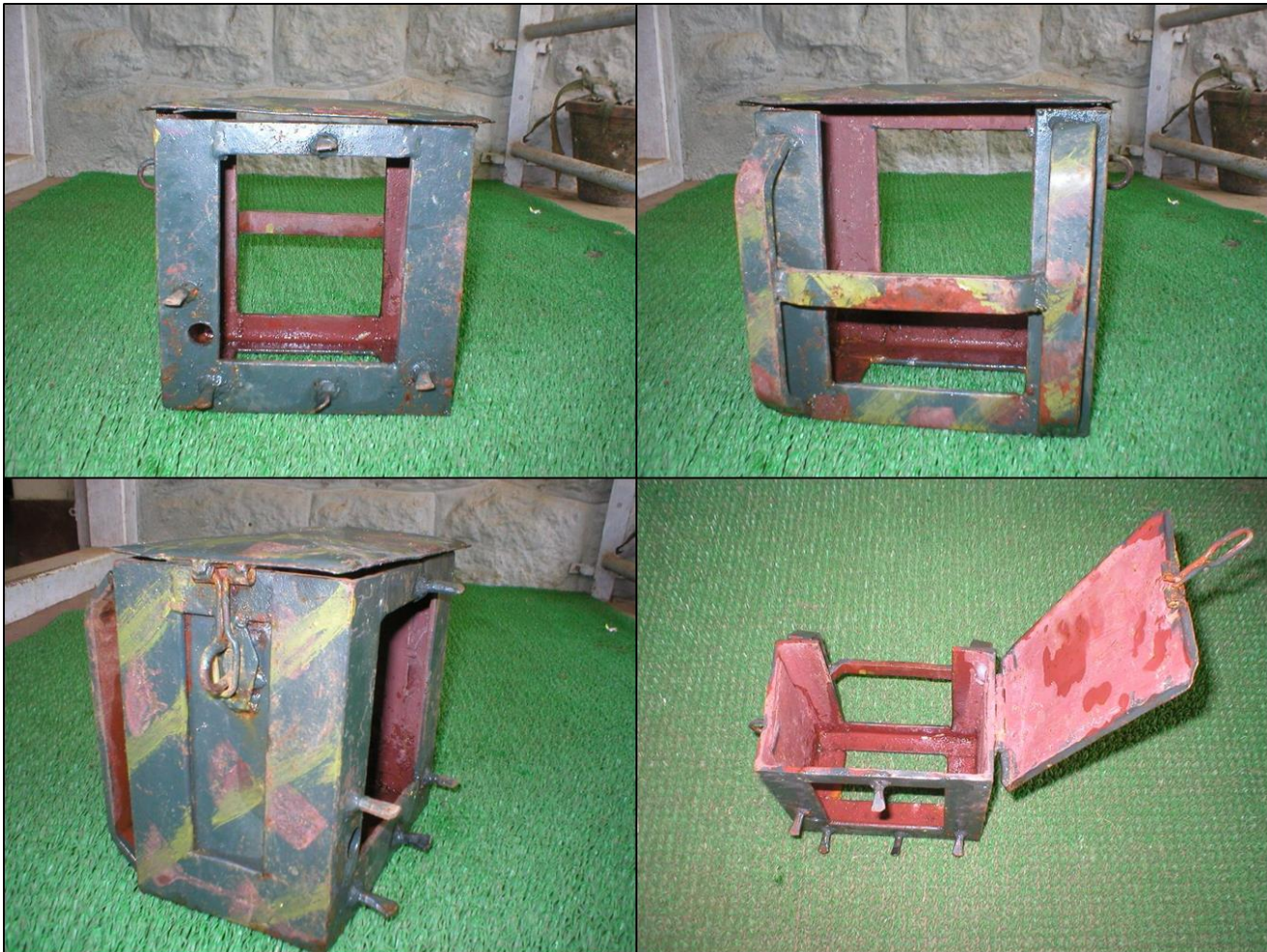
Figure 3.6 Design of metal case to secure camera traps from elephant damage and theft by people.
