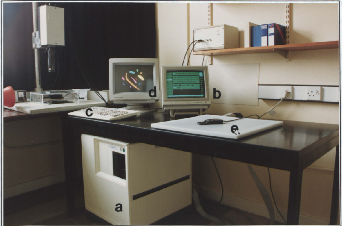
Figure 3.4 Photograph showing component parts of the image analysis system at Dunstaffnage Marine Laboratory. a) image processing unit and host computer, b) data monitor, c) keypad, d) colour monitor, e) digitizer tablet and mouse.
