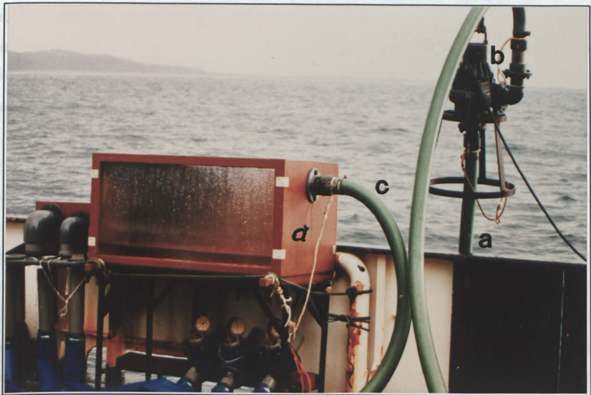
Figure 3.2 Photograph of the plankton pump used for sample collection on board the RRS Frederick Russell. a) intake hose, b) Flygt submersible pump, c) connecting hose, d) collecting tank, e) filter assembly, f) flowmeters.
