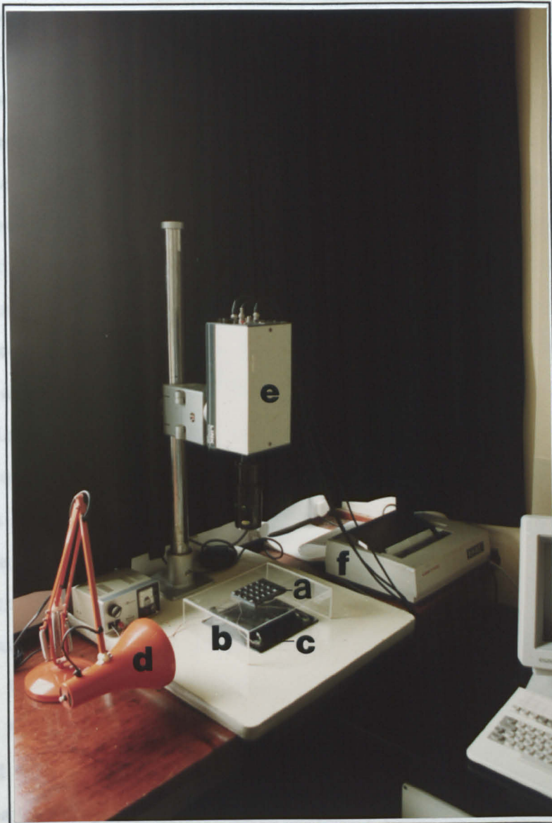
Figure 3.5 Photograph showing set-up used to process zooplankton samples by image analysis. a) sample tray, b) perspex table, c) LED light source, d) desk lamp, e) video camera, f) printer.
