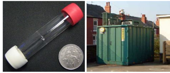
Figure 1: Nitrogen Dioxide diffusion tube vs. 'Groundhog' pollution automated station
