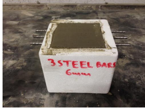
Fig. 2b. Mould with steel bars protruding (exposed) and top cover 5 mm.
