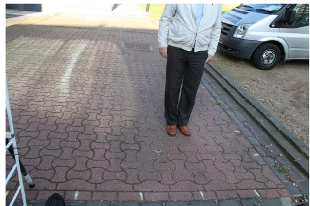
Figure 10. Outdoor arrangement for measurement of the intrusion detection probability. The volunteer was placed at all the nodes of the grid with the step of 0.5m.
