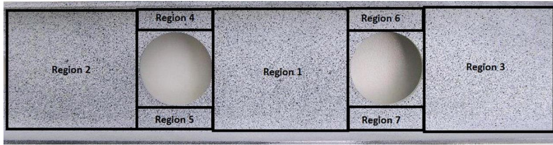
Figure 12: Division of the field in seven ROIs; ROIs 1, 2 and 3 have dimensions 60mmx50mm while ROIs 3, 4, 5, 6 and 7 have dimensions 35mmx12mm.
