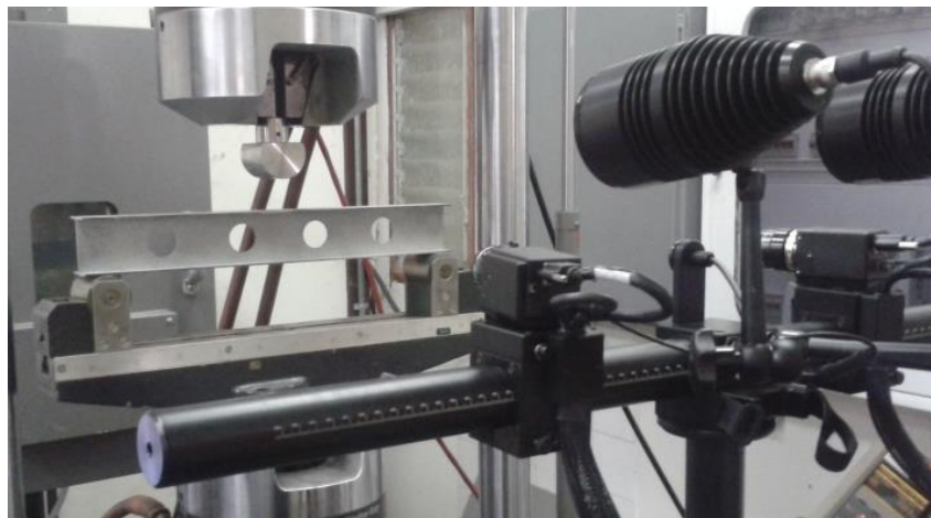
Figure 3: Experimental setup for testing of I-beam
