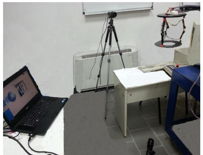
Fig. 9. Experimental set up for BAPAMAN1 with the CONTEMPLAS system.
