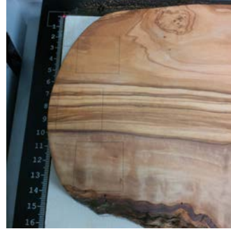
30 mm squares were laser etched into the wooden board to create a template for cutting out the stamp handles. As the wood was so thick and highly durable a bandsaw would be used to cut the board.
