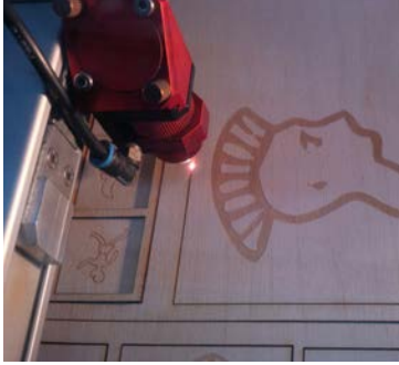
Various sizes of stamps templates were created on the lasercutter to assess what the size of the stamps should be.
