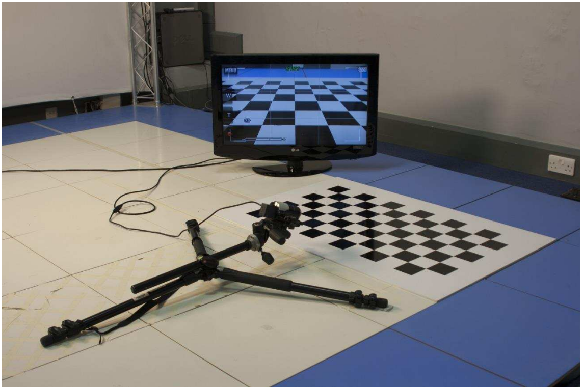
Figure 3.2. Experimental setup used to calculate calibration model error. A checkerboard scale swimming pool was used to calculate this error.
