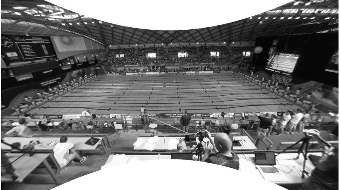
Figure 9.7. Undistorted image of the calibrated plane. Straight lines in the world, which were curved in the video footage, became straight in the undistorted image.
