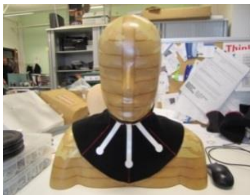
Figure 5. One of the development models of the Head Up neck orthosis for people with MND.
