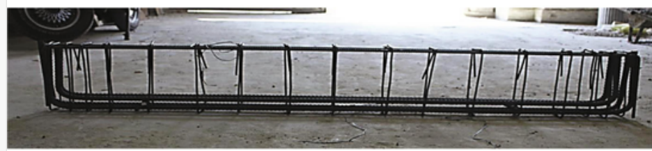
Beams with stirrups 7.5 Ø 6 /m
