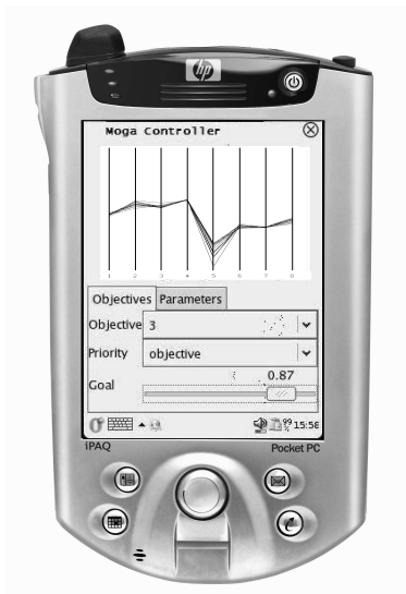
Fig. 6. A PDA Based Implementation of the Steering Client for our Multi-Objective Evolutionary Algorithm
