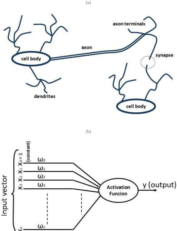
FIG. 1: (a) A neurone fires (or not) on the basis of the stimuli it receives from other neurones. (b) An artificial neurone weights the inputs it recesses and generates an output. It must be designed so as to produce the desired output.
