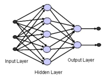
FIG. 2: Example of MLP with 3 units in the input layer, 5 units in the hidden (intermediate) layer and 2 units in the output layer.
