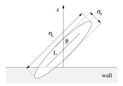
FIG. 3: The HNW potential: the molecules see each other (approximately) as uniaxial hard ellipsoids of axes  $(\sigma_0, \sigma_0, \kappa \sigma_0)$ , but the wall sees a molecule as a hard line of length L, which need not equal  $\kappa \sigma_0$ . Physically, this means that molecules are able to embed their side groups into the bounding walls. Varying L is therefore equivalent to changing the wall penetrability, which can be done independently at either wall.
