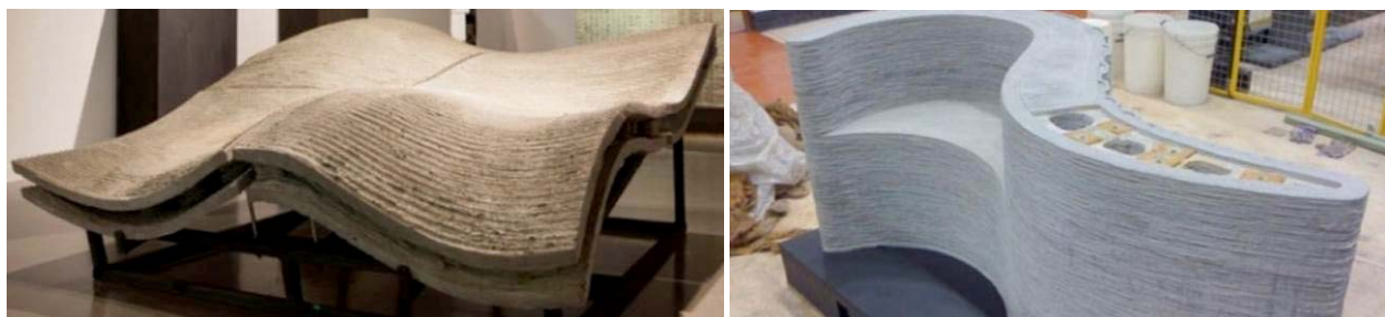
Figure 1. Free-form large scale concrete parts printed at Loughborough University (Le et al, 2012a; Le et al, 2012b; Lim et al, 2012)
