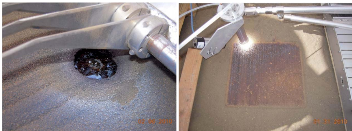
Figure 3. Melting of Tephra at 1800°C (left), and surface sintering at 1100°C (right) demonstrated through solar concentrator (Nakamura & Smith 2011)
