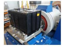
**Figure 10:** Mini-EUSO accomodation on the shaker - X direction
