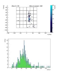
**Figure 3:** Top: UV Photon counts observed in the Mini-EUSO focal surface for a simulation of an  $E = 1 \times 10^{21}$  eV with an inclination of  $80^{\circ}$  to the nadir. Bottom: Light curve for the same event as a function of time in units of GTU (1 GTU =  $2.5\mu$ s). [11]
