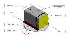
**Figure 9:** Mini-EUSO Vibration set-up scheme for Z axis
