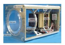
**Figure 4:** Telescope mechanical body with subsystems.
