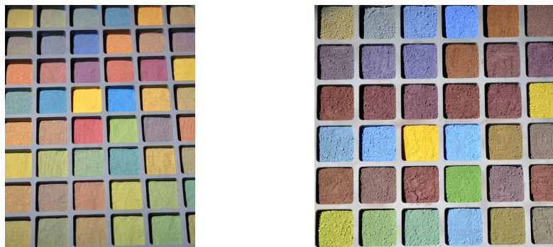
Figure 5. Images of quartz sands (left) and colour powders (right) in boxes to be captured by our hyperspectral camera.
