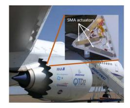
Figure 3.9: Chevron with SMA actuators for noise reduction during flight take-off [101].
