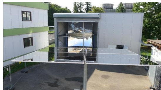
Figure 1: Solar furnace arrangement consisting of a heliostat mirror (front, outside) and a parabolic mirror (back, inside the laboratory) (Foto: J. Flesch).
