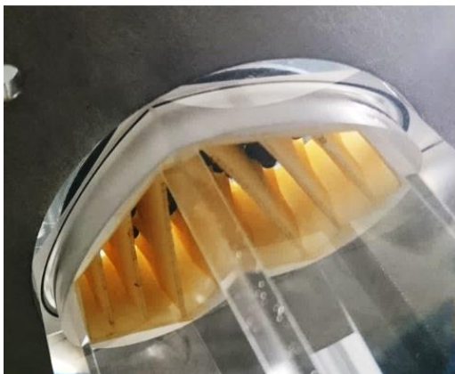
Figure 5a: 19 particles of 3.0mm diameter in the pin fixer
