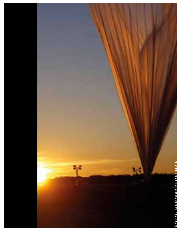
Measurement of stratospheric substances: Balloon, whose gondola carries a unique combination of remote sensing instruments, shortly before launch
