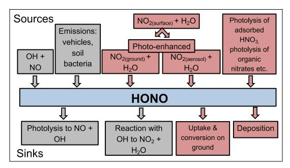
**Figure 12.** Diagram of major HONO sources and sinks in the troposphere. Boxes in gray represent the traditionally understood sources and sinks, and boxes in red show more recently established processes (see text for references). DOI: https://doi.org/10.1525/elementa.2020.034.f12
