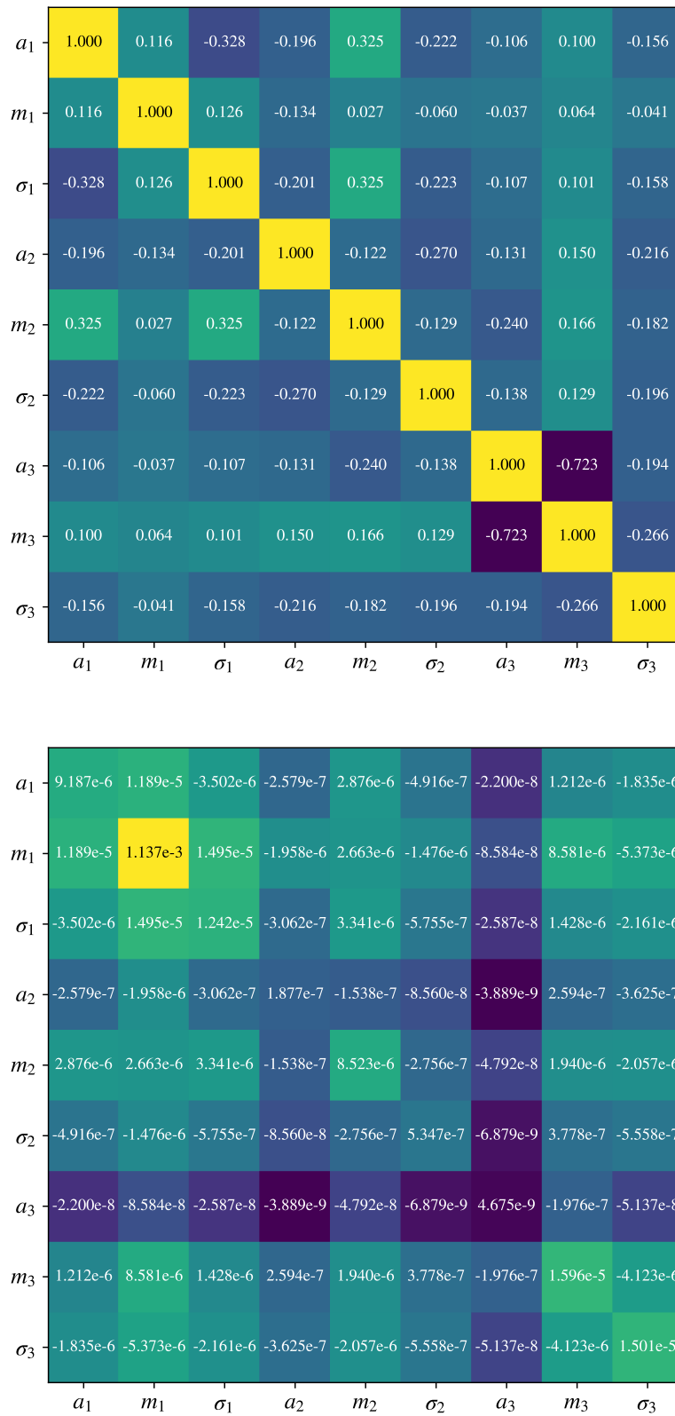
Figure A.2: Correlation matrix (top) and covariance matrix (bottom) for the energy-loss function parameters in Tab. A.1 as obtained from the combined \chi^2 fit using only integral response functions for molecular tritium.
