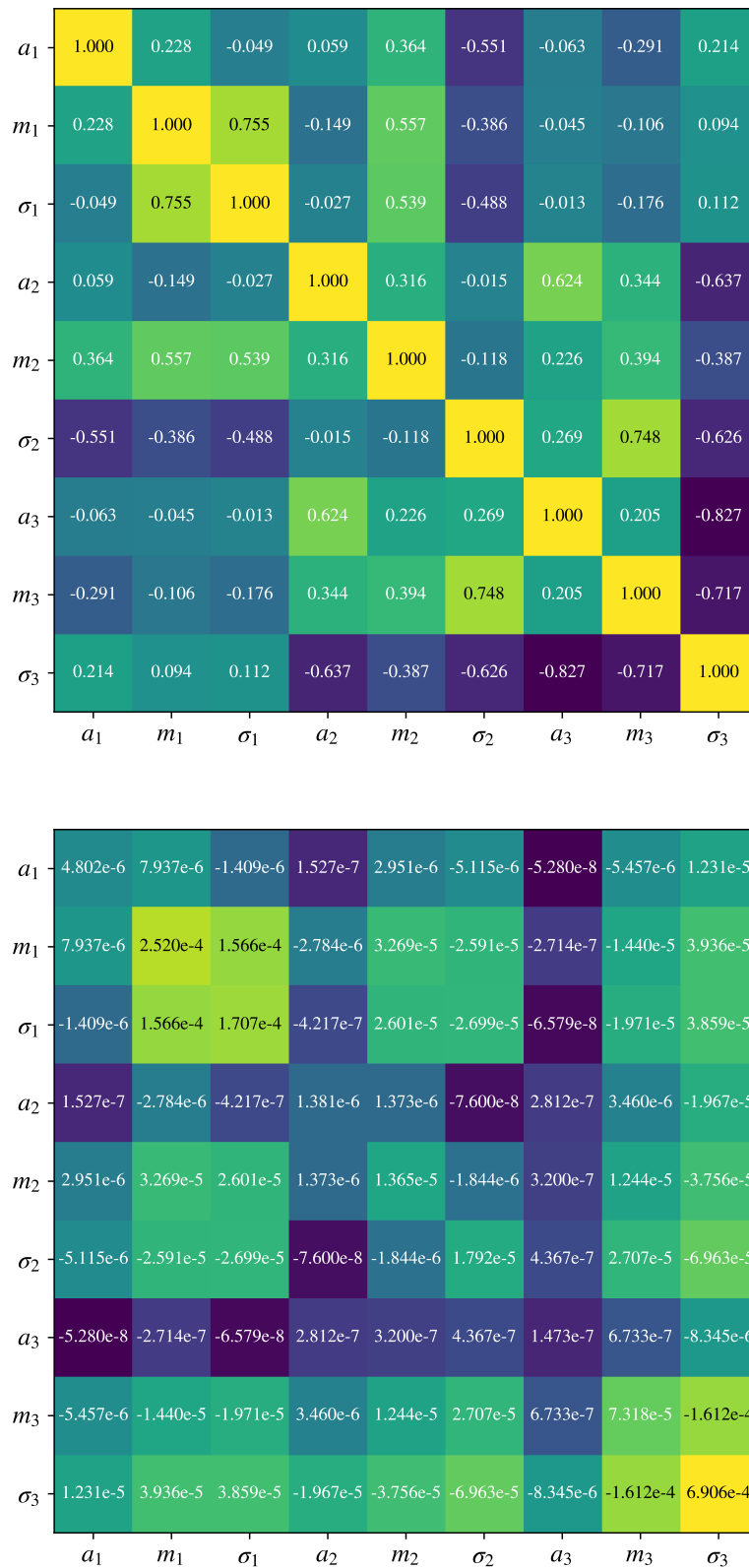
Figure 7.16: Correlation matrix (top) and covariance matrix (bottom) for the energy-loss function parameters in Tab. 7.5 as obtained from the combined \chi^2 fit to integral and differential response functions for molecular deuterium.
