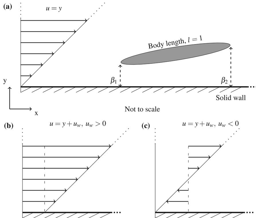
**Fig. 8** Sketch of the body situated near the wall within uniform-shear flow parallel to the wall with the typical gap width. **a** Zero wall velocity relative to the body. **b** Positive wall velocity relative to the body. **c** Negative wall velocity relative to the body
