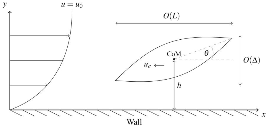
**Fig. 1** Diagram showing the set-up for Sect. 2: a thin body translates with speed  $u_c$  in the boundary layer of a much larger body, which acts as a stationary wall. The distance of the body’s centre of mass (CoM) from the  $x$ -axis is  $h$  and the angle its chord line makes with that axis is  $\theta$ . The incoming velocity profile (due to the motion of the larger body) is  $u = u_0(y)$
