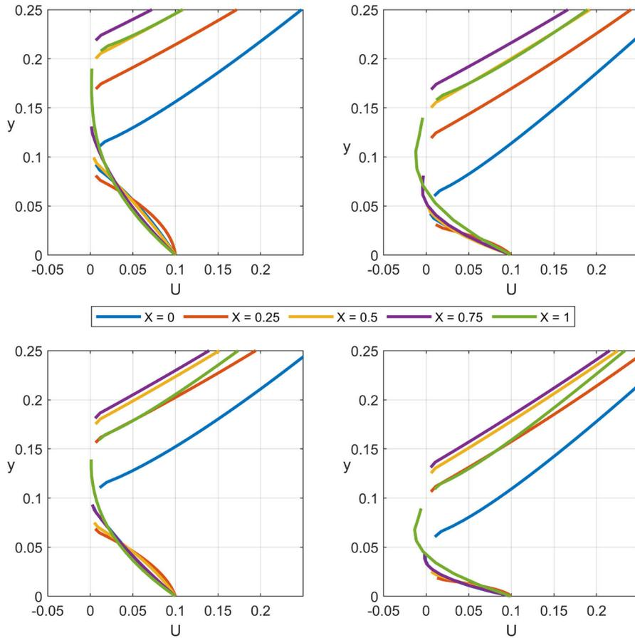
**Fig. 9** Velocity profiles underneath and on top of the body taken at various points for  $u_w = 0.1$ . Flow reversal is seen along the body as the leading edge gap  $\beta_1$  decreases. Top row, left:  $\beta_1 = 0.1$  and  $\beta_2 = 0.2$ , Top row, right:  $\beta_1 = 0.05$  and  $\beta_2 = 0.15$ . Bottom row, left:  $\beta_1 = 0.1$  and  $\beta_2 = 0.15$ , Bottom row, right  $\beta_1 = 0.05$  and  $\beta_2 = 0.1$  (right)
