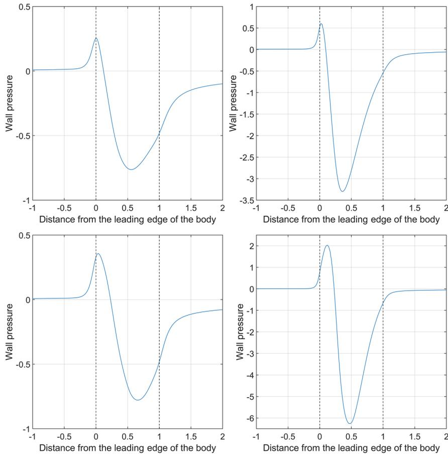
**Fig. 11** Profiles of the pressure along the length of the wall for  $u_w = 0.1$ . Top row, left:  $\beta_1 = 0.1$  and  $\beta_2 = 0.2$ , Top row, right:  $\beta_1 = 0.05$  and  $\beta_2 = 0.15$ . Bottom row, left:  $\beta_1 = 0.1$  and  $\beta_2 = 0.15$ , Bottom row, right  $\beta_1 = 0.05$  and  $\beta_2 = 0.1$  (right)
