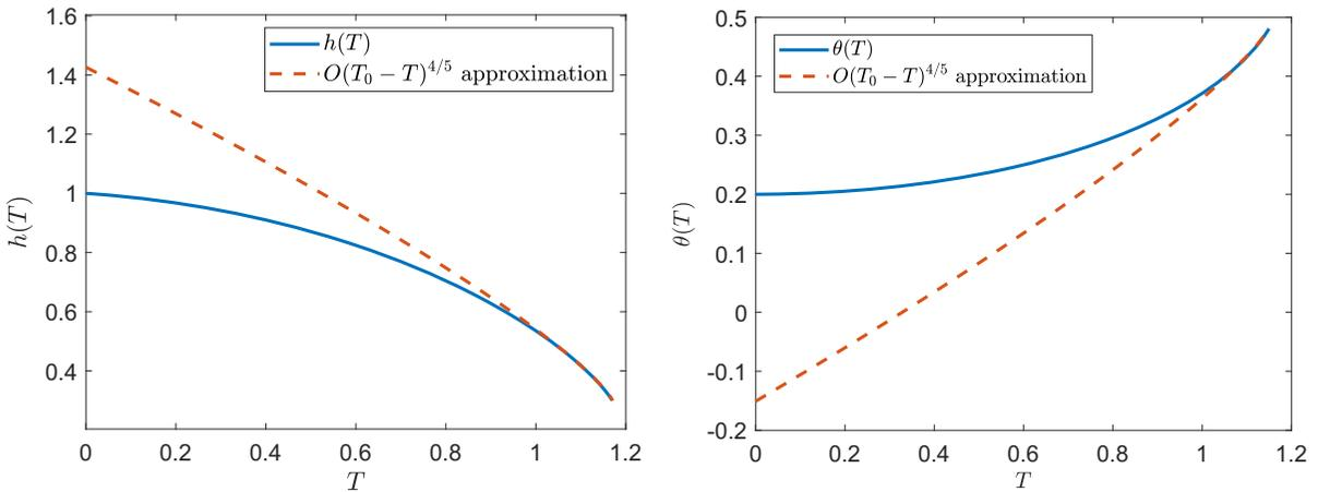
**Fig. 2** Numerical solutions of  $h$  and  $\theta$  for a body with  $M = 1$ ,  $I = 0.2$  are shown in solid blue, with incoming flow profile  $u_0 = 2 - \exp(-Y)$ . Initial conditions were  $h(0) = 1$ ,  $\theta(0) = 0.2$ ,  $h_T(0) = -0.1$ ,  $\theta_T(0) = 0$ . The dashed red curves vary as  $(T_0 - T)^{4/5}$  with the end points fixed to match the corresponding  $h$  or  $\theta$  value there
