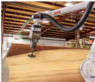
Figure 1.1: A robot sanding a surface [Rob21].
