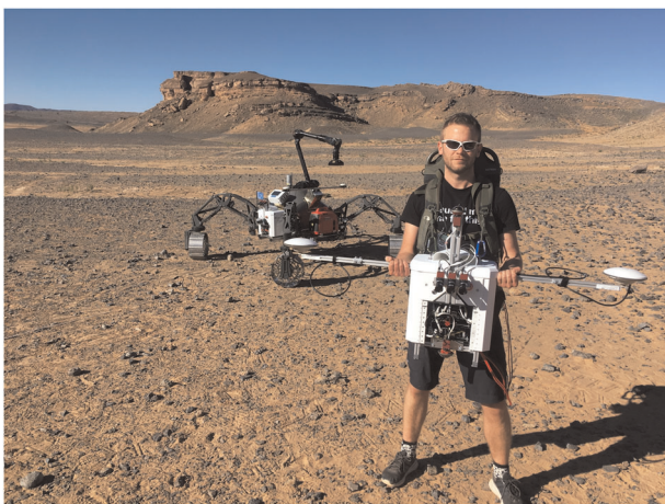
FIGURE 1 The two SUPER units in the Moroccan desert on the Rissani 1 location: One unit is mounted on the SherpaTT rover (Cordes et al., 2018) of the DFKI Robotics Innovation Center (background) and the other is used as human-carried device (foreground). The data presented in this article were captured by the hand-held device [Color figure can be viewed at wileyonlinelibrary.com ]
