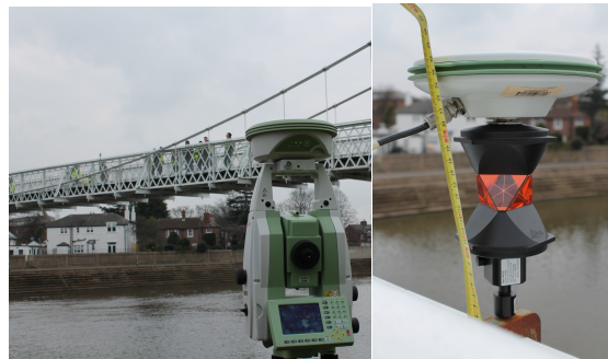
Fig. 2: The RTS with the GPS station for recording in GPS time (left) and the GPS antenna with the reflector mounted on the handrail at the midspan of the bridge (right).
