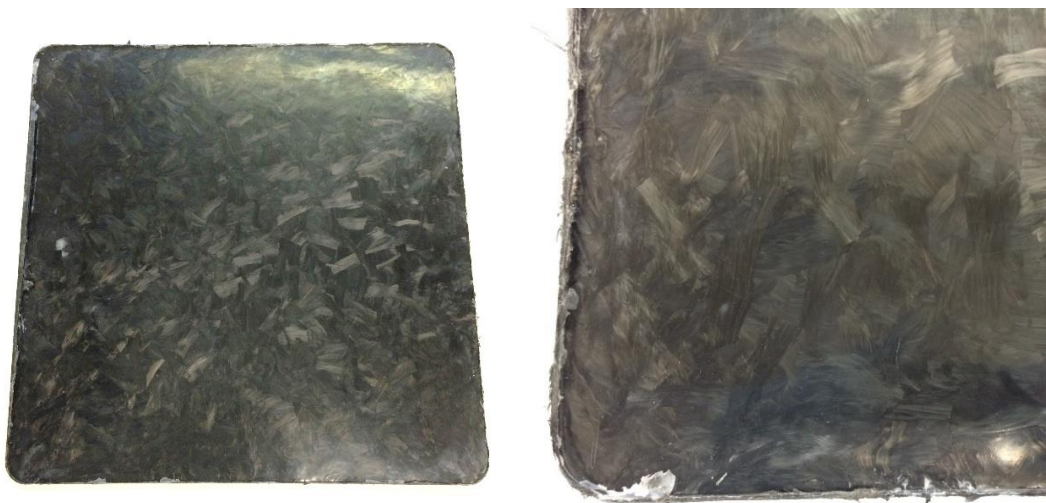
Figure 3-17 - Carbon Fibre/Polypropylene panel moulded at 0.45V f manufactured using NI-CM for this study
