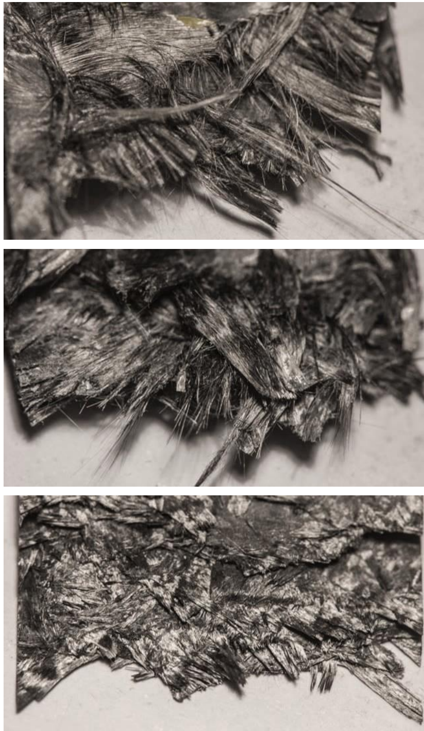
Figure 6-1 – Tensile fracture sites of CF.PP (top), CF.mPP (middle) and CF.EP (bottom) all moulded at 0.45V_f
