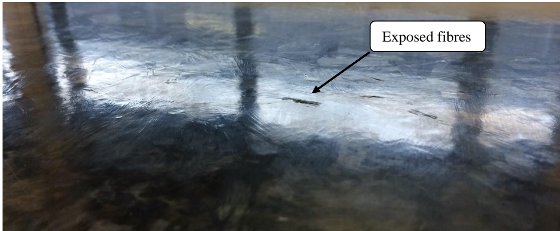
Figure 6-7 – Exposed fibres on the surface of a moulded panel due to local variations in volume fraction
