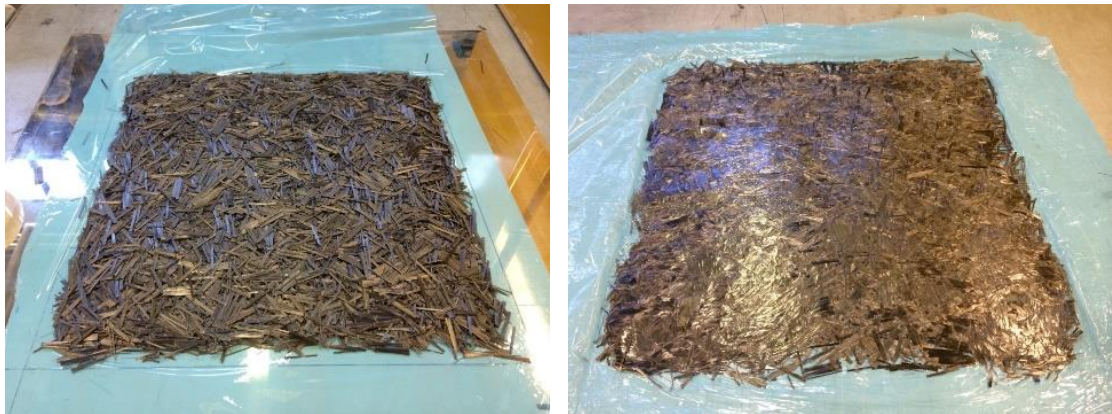
Figure 3-15 - Preforming for 406mm square parts. Fibre stack before preforming (left) and fibre stack after preforming (right)
