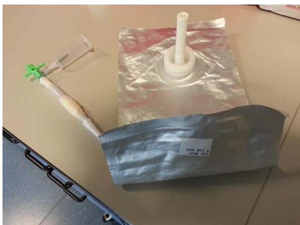
Figure 2.7: Breath bag and 3 way-tap to collect breath samples for ^{13}\text{CO}_2 analysis
