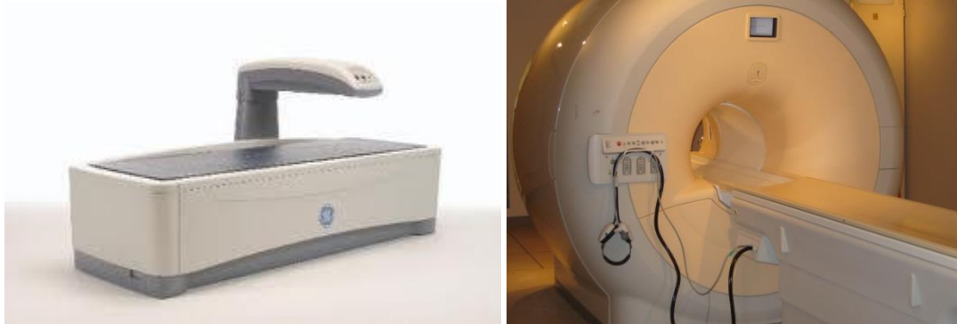
Figure 2.10a and b: DEXA scanner and MRI scanner used to determine body composition in Studies 1, 2, 4 and hepatic and muscle triglyceride in study 3 respectively.
