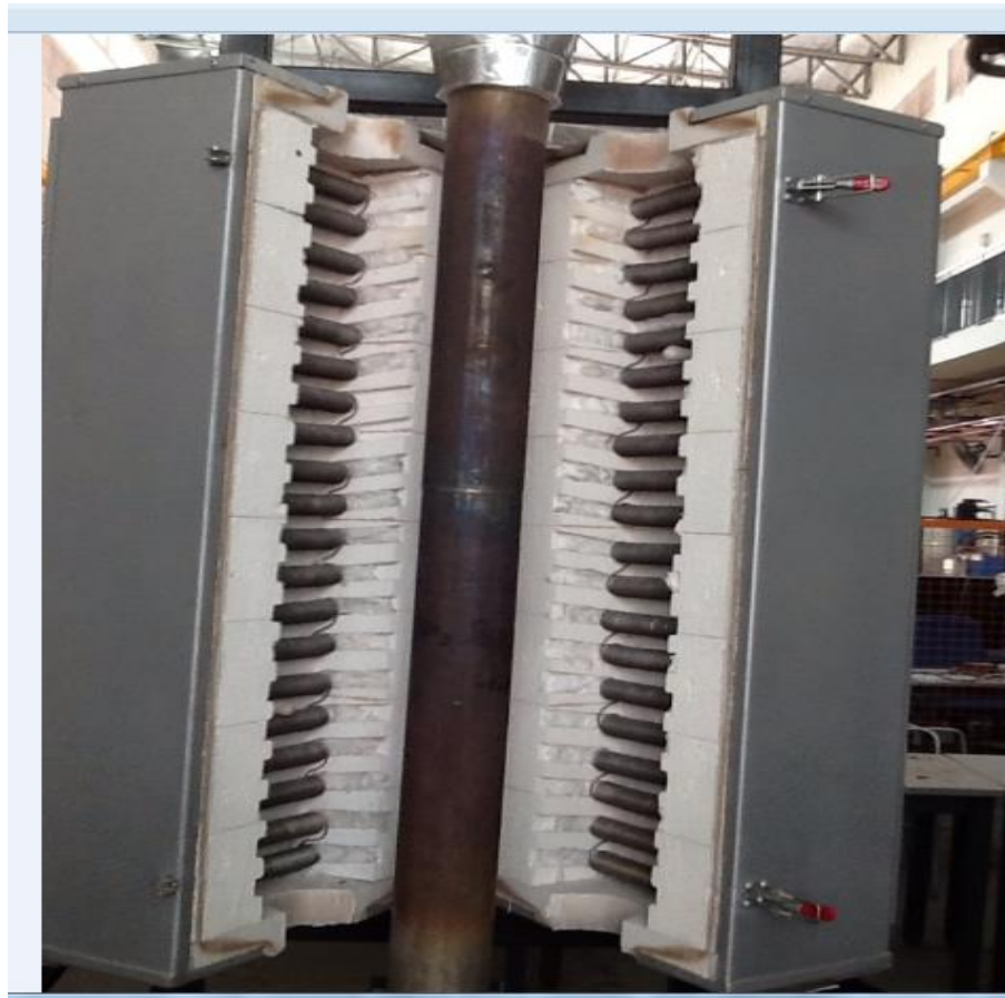
Figure 3-5: Picture of the vertical split jacket heater and reactor tube
