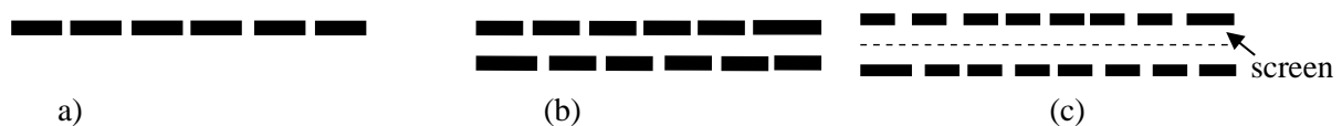
Figure 2-16: Various types of perforated plate distributor configurations: (a) single plate distributor, (b) double plate distributor, (c) screen sandwiched double plate distributor (Kunii and Levenspiel, 1991).
