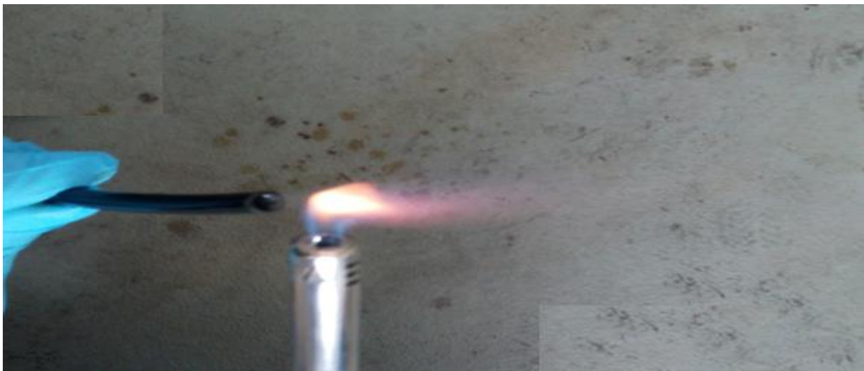
Figure 6-5b: The flame of lighter after the syngas is passed on it (the syngas changes the colour of the flame as it is burning).
