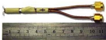
Fig. 3.13. Fabricated E-field probe [21].
