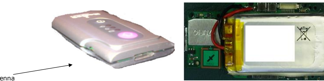
. PCB with a Bluetooth Module.
