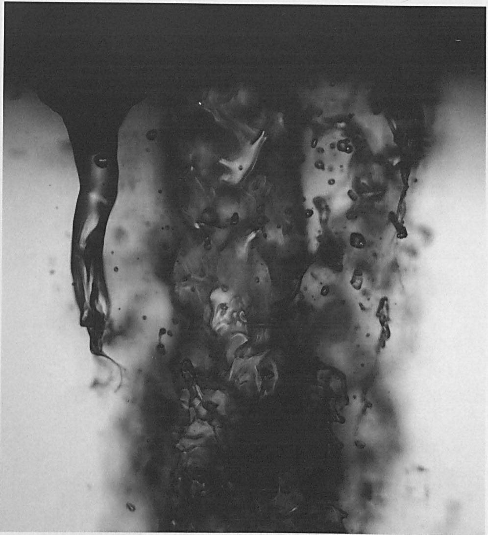
Figure 5-17: Liquid core at exit of nozzle, FOV 1028 x 1076 px (1.41 x 1.48 mm), \Delta t = 100\text{ns}
