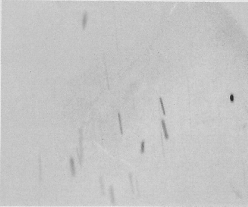
Figure 5-6: Streaks due to motion blurring of liquid droplets
