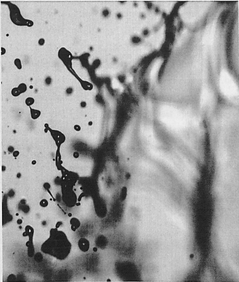
Figure 7-2: Water sheet breakup in impact pin nozzle (top) FOV 1197 x 1080 px (1.65 x 1.49 mm) \Delta t = 100\text{ns} (bottom) FOV 951 x 1080 px (1.31 x 1.49 mm) \Delta t = 100\text{ns}
