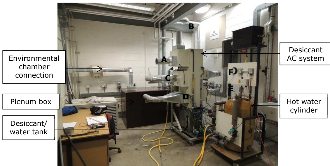
Figure 5-7 IDCS laboratory setup with labelled air flows
