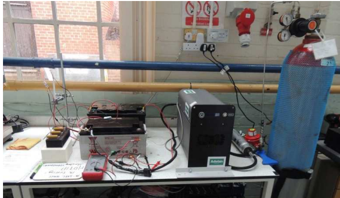
Figure A4-1 UoB micro-tubular SOFC test set-up
