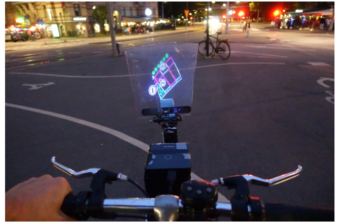
Figure 3. Map navigation using a bike-mounted head-up display. The navigated route is shown in pink. Landmarks are highlighted.
