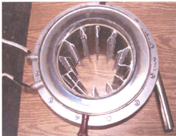
Figure 3-3 Purposefully designed fuel-powered furnace for central heating system integrated with thermoelectric generation [131]
