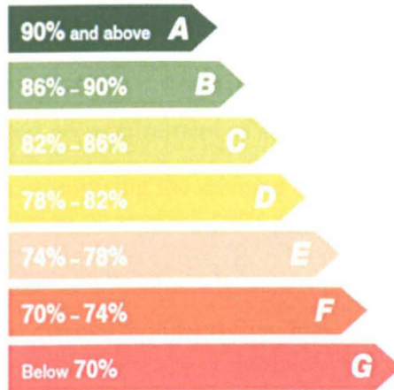
Figure 4-4 Rating chart of domestic boiler by SEDBUK
