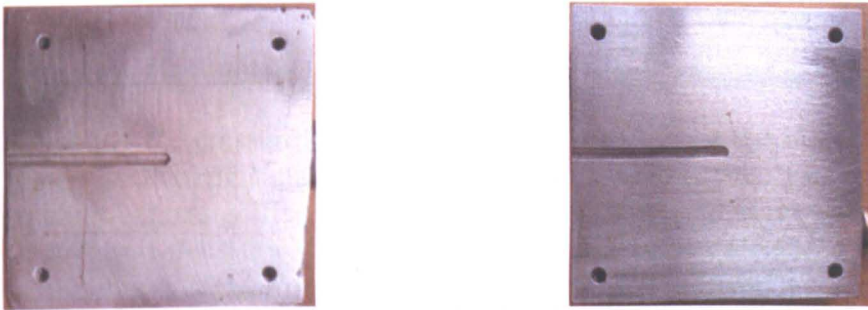
Figure 5-42 Slots on the heat exchangers for the thermocouples (left to right: hot side, cold side)
