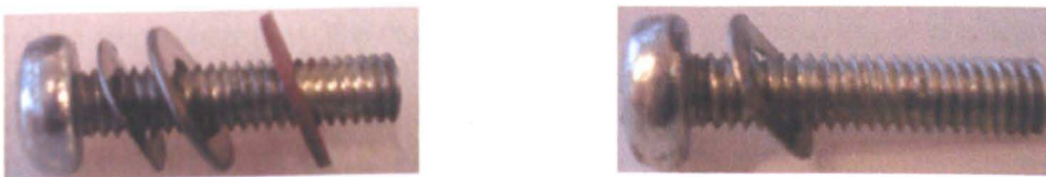
Figure 6-32 Washer configurations in the assembling procedure (from left to right, crinkle washer, flat metal washer and fibre washer)
