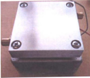
Figure 5-8 The photo and schematic diagram of the single thermoelectric cogeneration block
