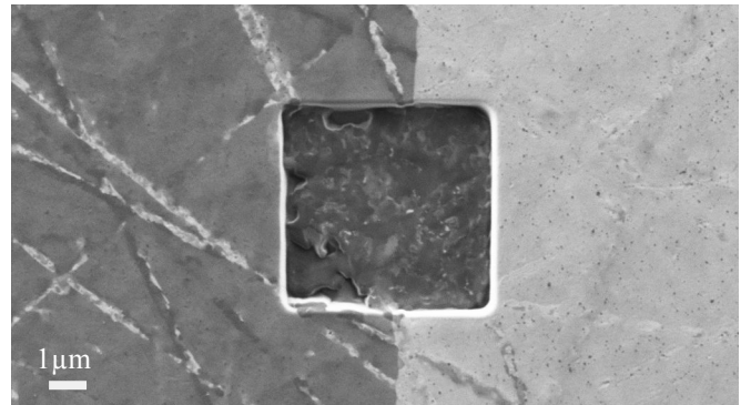
Fig.5: Channelling contrast FIB image of pattern milled at the boundary of two grains
