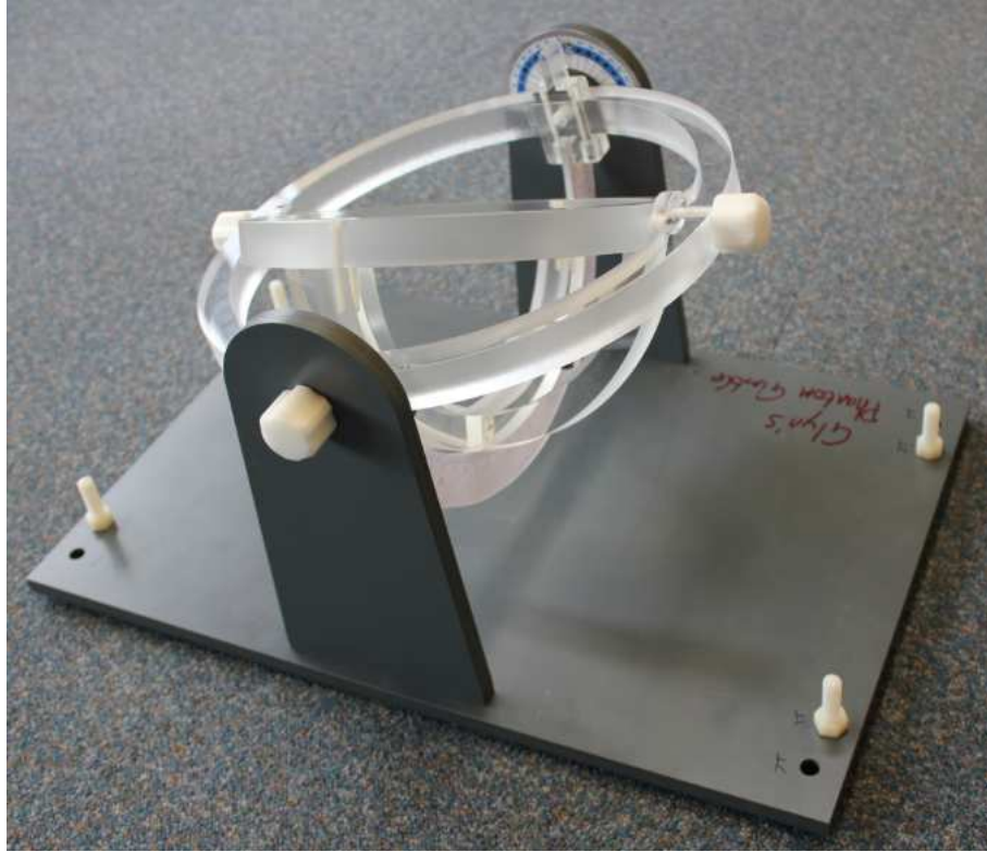
Figure 6.4: A custom gimbal for rotating the spherical phantom within the bore of the MRI scanner.
