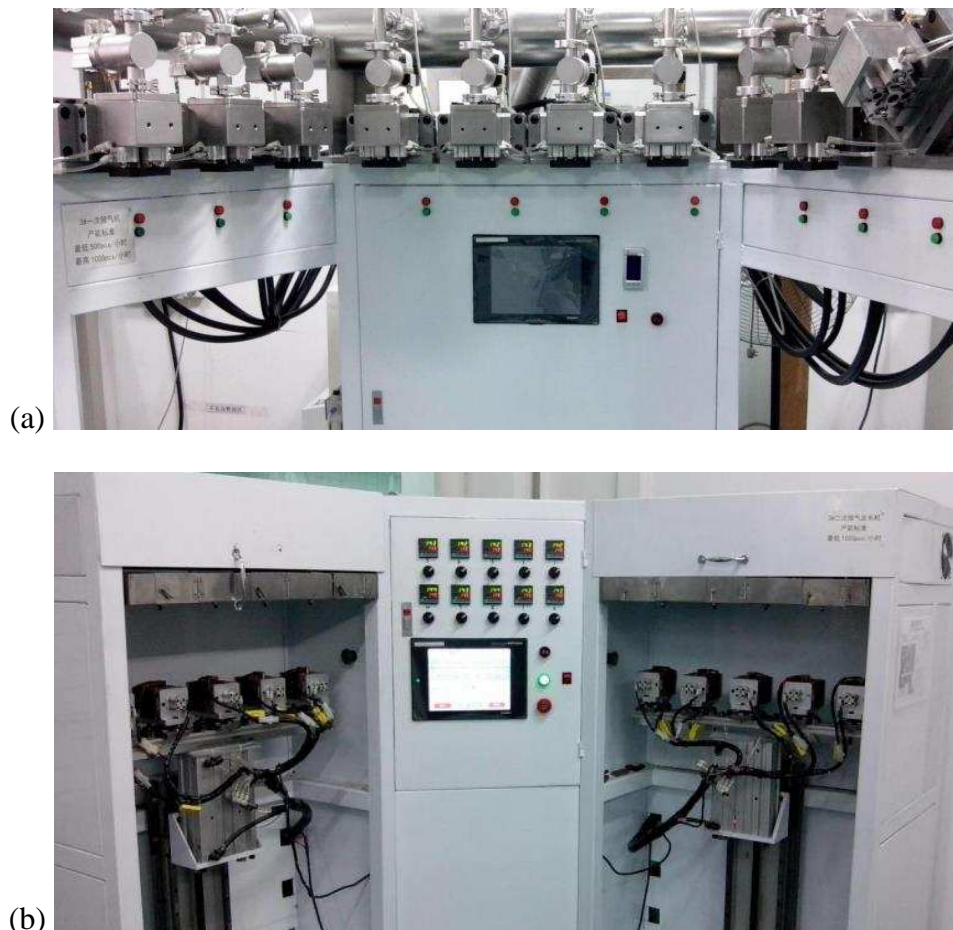
Figure 7.24: Fabrication in process – (a) 1 st degassing equipment; (b) 2 nd degassing equipment.
