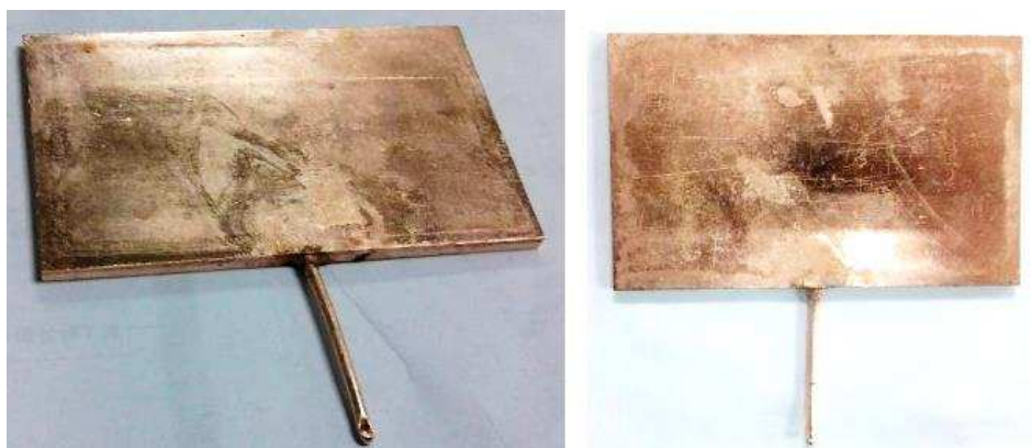
Figure 7.22: Fabrication in process – product after inserting tail pipe and welding.
