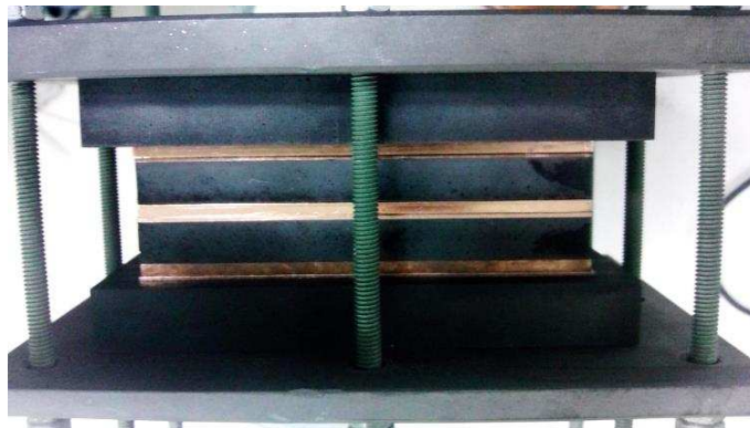
Figure 7.20: Fabrication in process – holding sintered upper and bottom plates.
