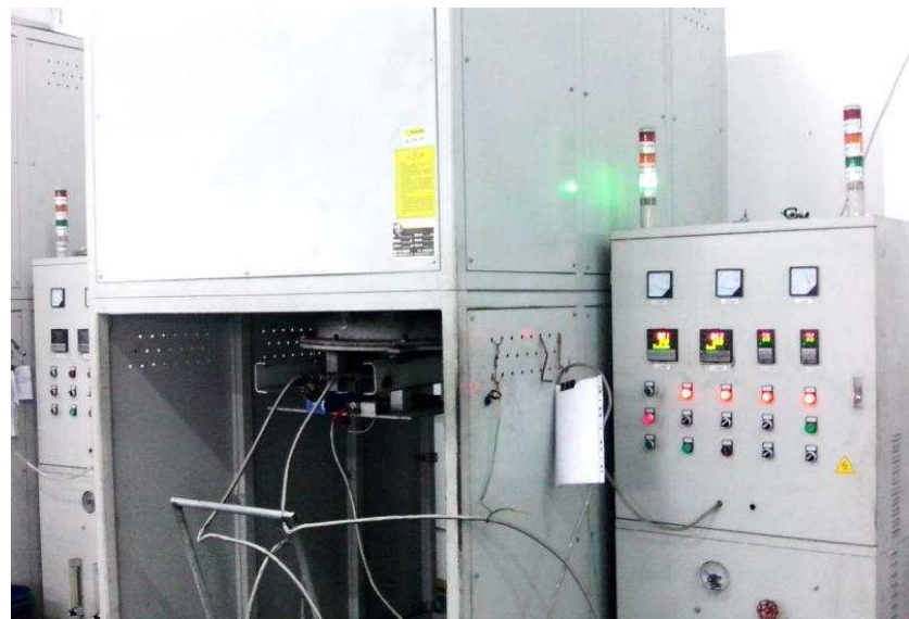
Figure 7.18: Fabrication in process – furnace sintering.
