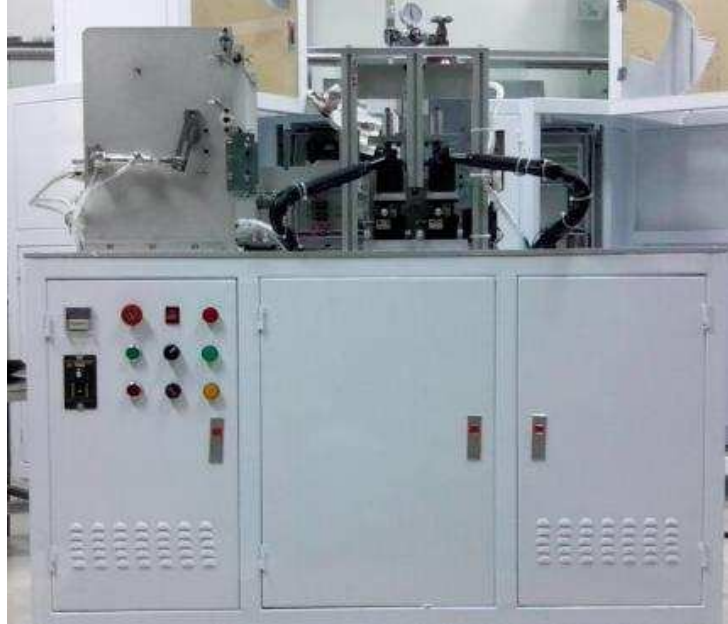
Figure 7.25: Fabrication in process – TIG welding machine.
