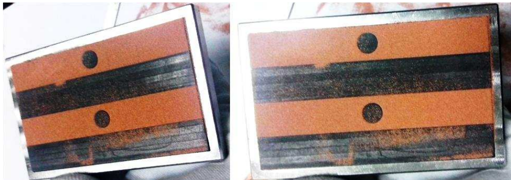
Figure 7.16: Fabrication in process – powder filling.
