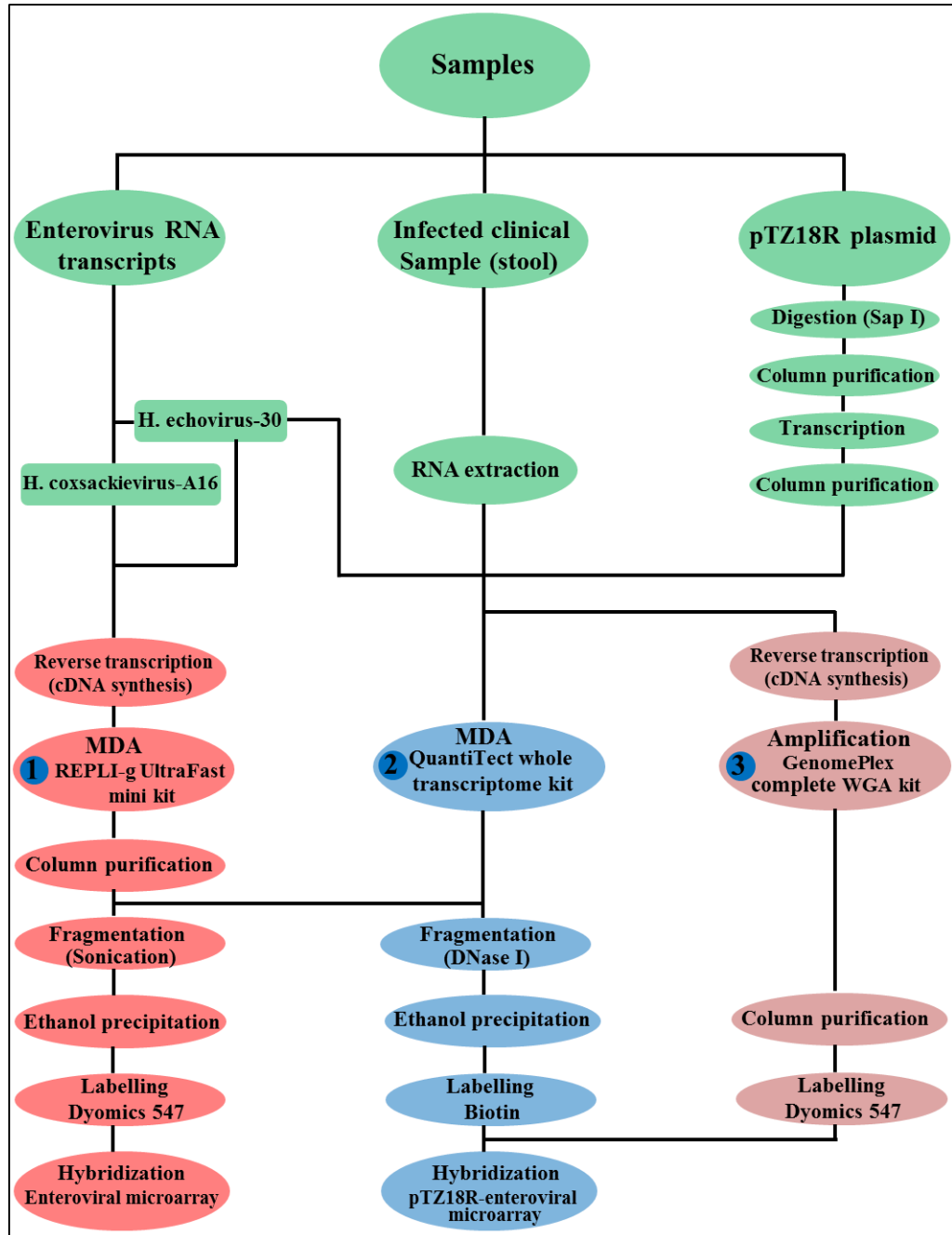
Figure 3-26: Schematic diagram showing the steps used for optimizing hybridization process using the experimental microarrays.
