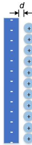
Fig. 2.6 Schematic representation of the double layer. d is the thickness of the double layer.
