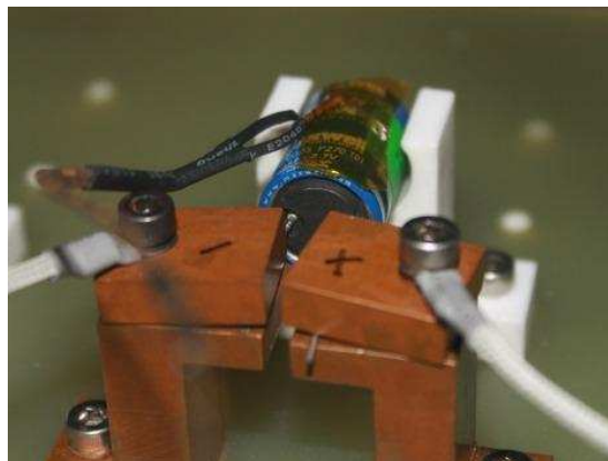
Fig. 3.9 K-type thermocouple attached on supercapacitor surface for temperature measurement.
