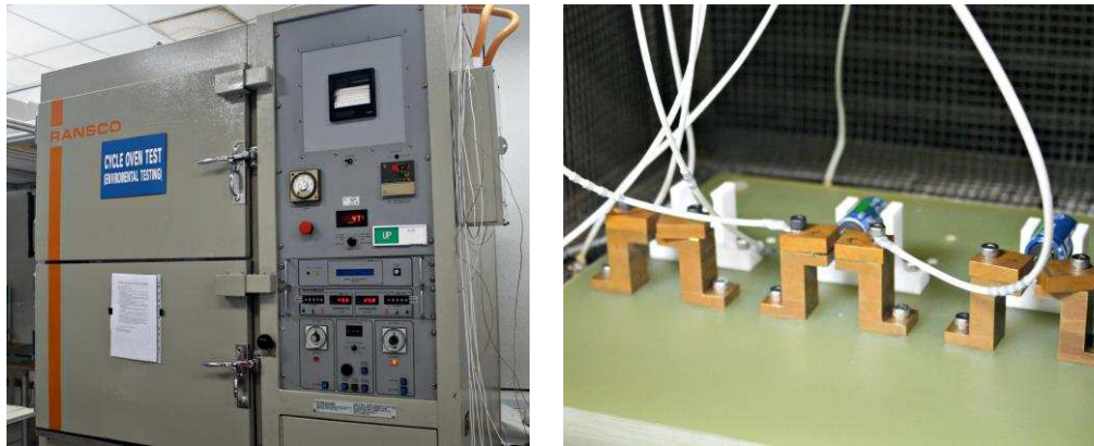
Fig. 1.6 Test bench of the experiment: RANSCO Environmental Chamber used to perform the accelerated ageing test (left) and inside view of the environmental chamber shows a fibre glass tray with supercapacitors mounted on top. Each supercapacitor is connected to a separate current source (right).
