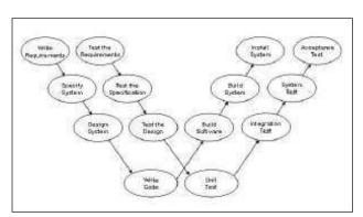
Figure 30 The W-Model of testing [241]
