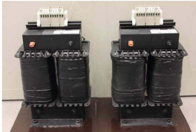
Figure 7.3: A photograph of the two isolation transformers.
