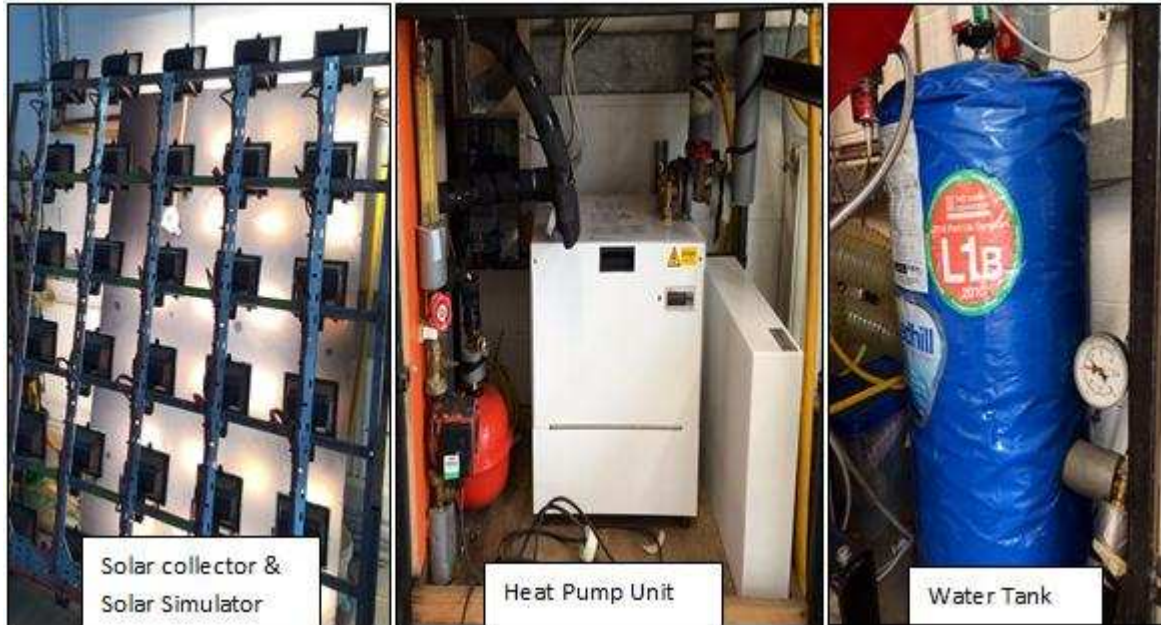
Figure 7.2.3 Experimental Design - Novel Solar Thermal roof with Solar Simulator, Heat Pump, Water Storage
