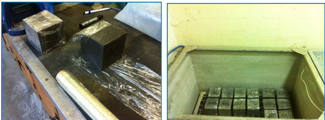
Figure 3-9 Sealed curing (wrapped in cling film)
