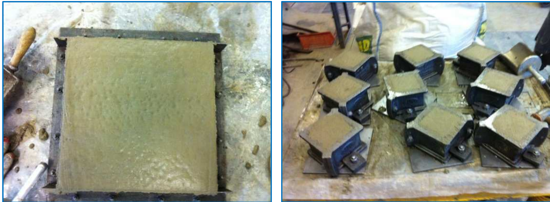
Figure 3-7 Moulding process of cubes and slab specimens
