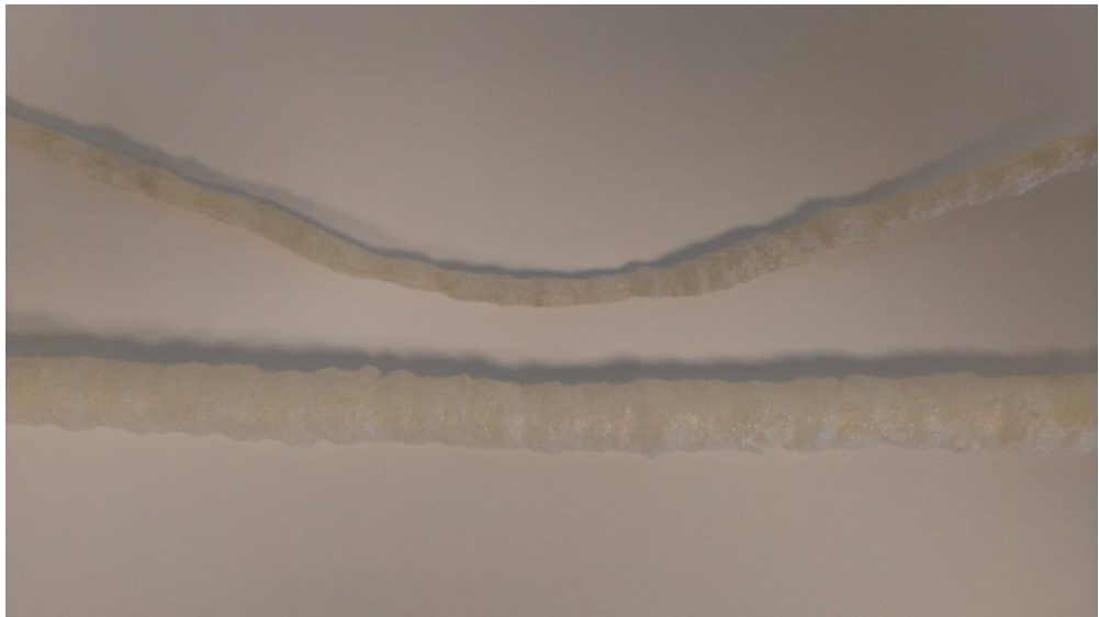
Figure 4.27 Extruded foams of 70 wt% starch + 30 wt% CF (top) and pure starch (bottom).
