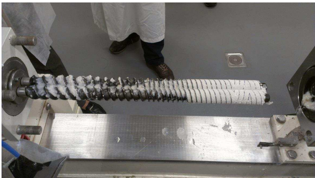
Figure 4.21 The extruder screws became blocked as the cellulose dried towards the end of the barrel.
