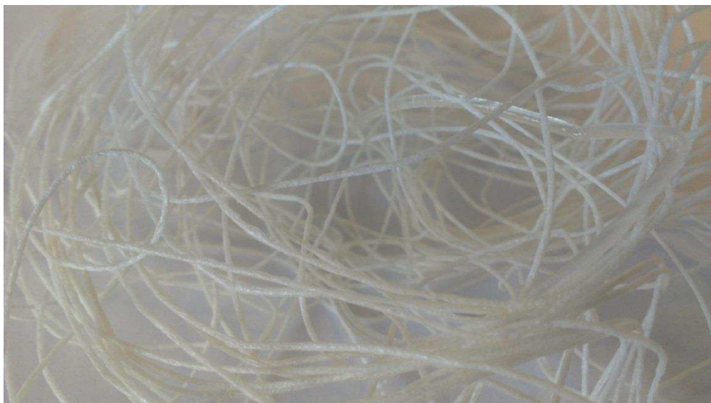
Figure 4.32 70 wt% HPC + 30 wt% MCC extrudate from the capillary rheometer using a 0.5 mm diameter capillary die.
