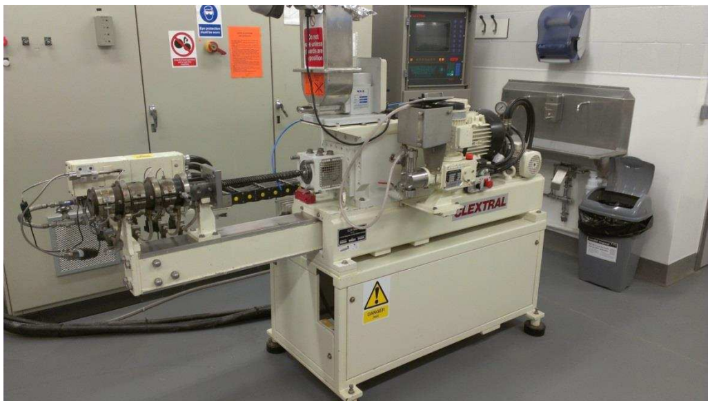
Figure 4.20 The Clextral extruder used for the initial fibrillation experiments.
