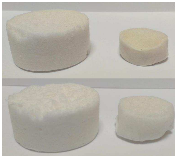
Figure 4.16 Foams at 97% RH LBG (top) and fenugreek (bottom) with pure galactomannan on the right and galactomannan + CF at a ratio of 1:4 on the left.
