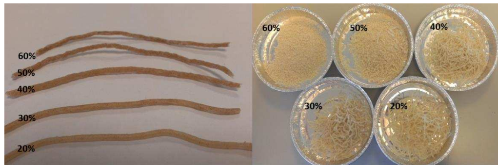
Figure 6.5 LBG (left) and fenugreek (right) extruded from a capillary rheometer. Numbers next to each sample represents the concentration of polysaccharide.
