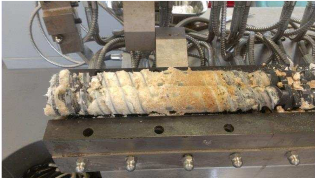
Figure 4.25 The screws of the extruder became blocked at low water flow rates.
