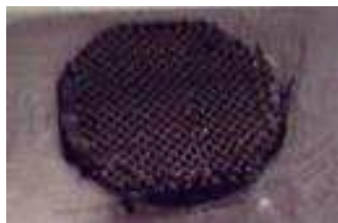
Fig. 4.5: ACTS fabric specimen before the through thickness permeability K_3 measurement.
