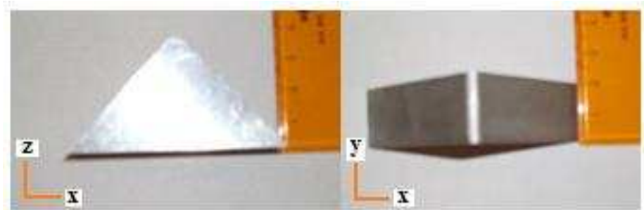
Fig. 3.8: Aluminium curve plate xyz axis 48 \times 19 \times 39 mm used for bending tests.
