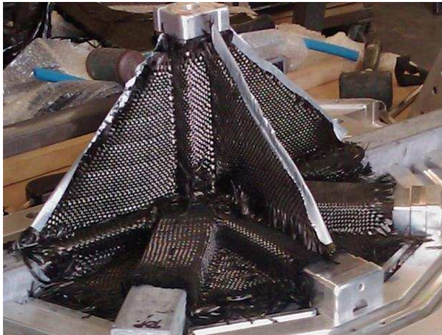
Fig. 7.9 (b): Analysis of fibre orientations, right side view.
