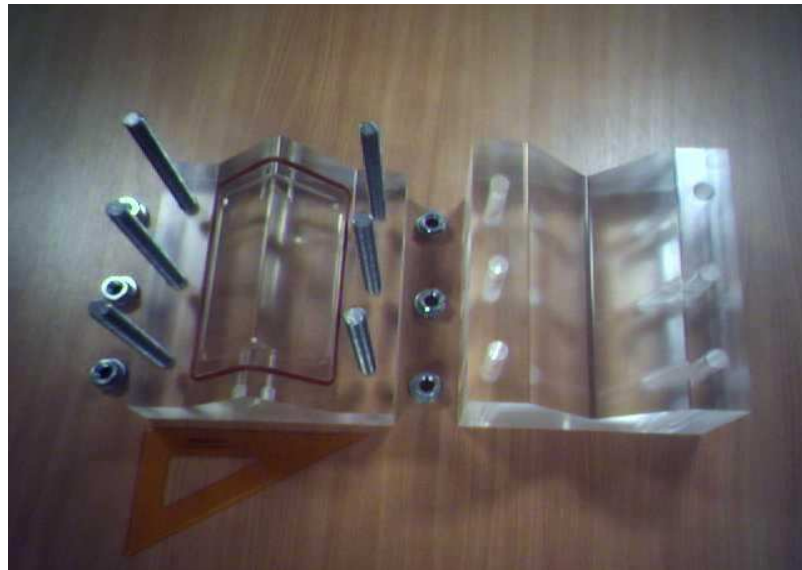
Fig. 6.1: Transparent tooling (male left, female right) for the race-tracking study with a 90^\circ curved plate. The cavity dimensions for the male part were: 150 \times 150 \times 2.75 mm.
