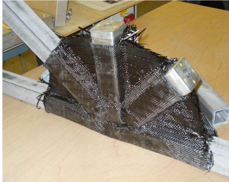
Fig. 1.3: ACTS generic node preform with HTS40 F13.
