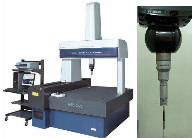
Fig. 3.11: Mitutoyo coordinate measuring machine, with scanning probe, (right).
