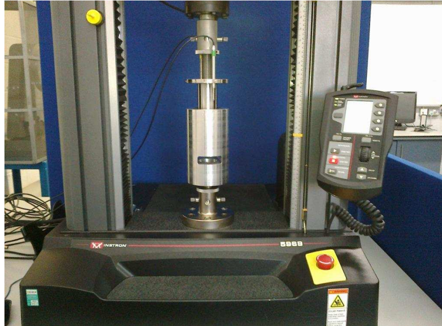
Fig. 3.1: Compaction testing rig.
