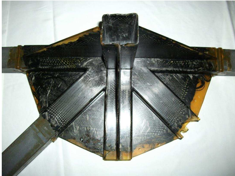
Fig. 9.3 (a): Prototype manufactured node top surface view.
