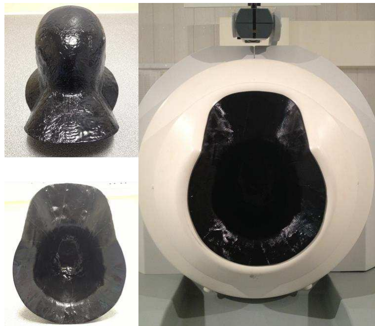
Figure 2.9: The fibre glass insert created to line the MEG helmet.
