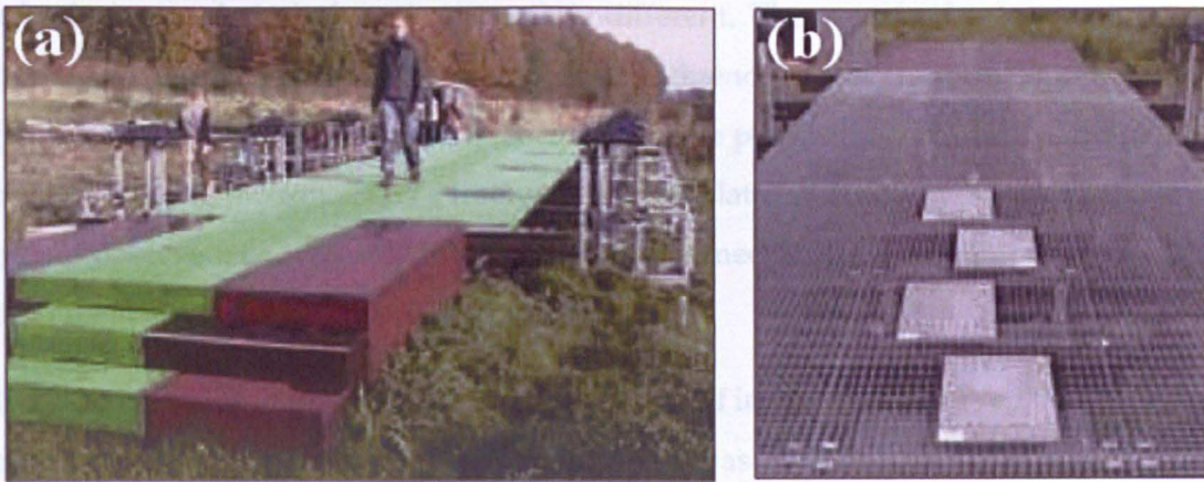
Figure 2.22: Plot (a), 12 m \times 3 m platform employed by Butz et al. Plot (b), 4 load cells measuring 0.4 m \times 0.6 m embedded in the walkway, after [9].
