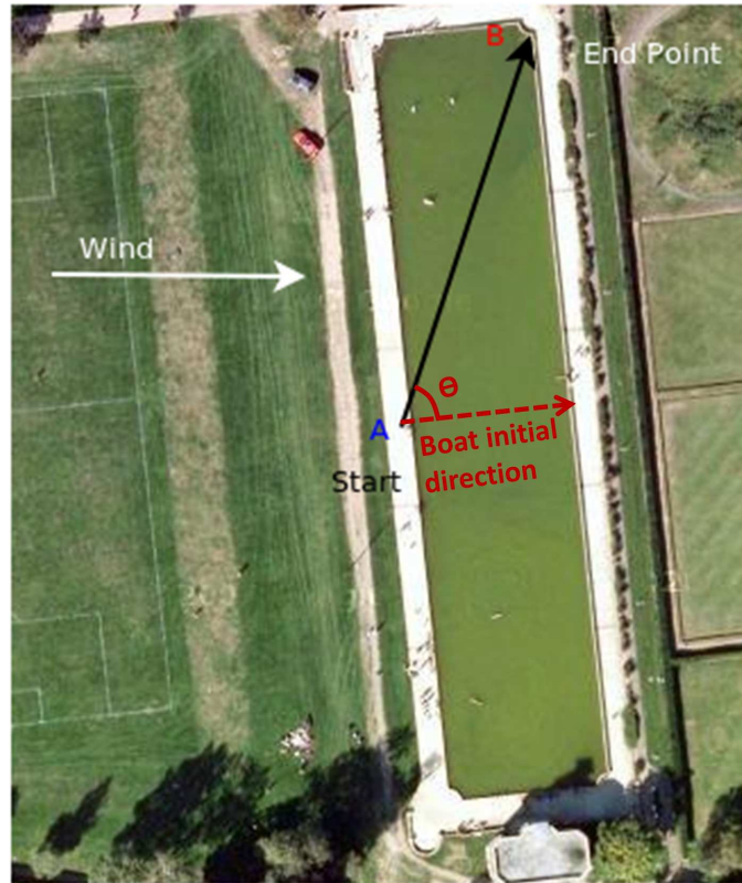
Figure 6.5: Modified boat course including newly added turn indicated by \theta . Start point is shown by 'A' and end point shown by 'B'
