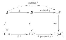
The left square commutes by assumption while the right square commutes because unfold g is a coalgebra homomorphism. Therefore, the outer rectangle commutes, meaning that unfold  $g \circ h$  is a homomorphism from f to *out*. Finally, because homomorphisms to the final coalgebra *out* are unique and unfold f is also such a homomorphism, the result unfold  $g \circ h =$  unfold f holds.
